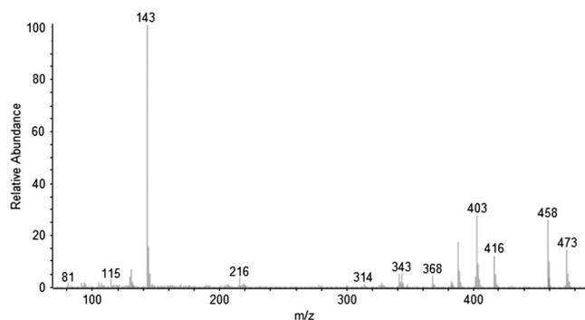
**Figure 2.** Full Scan GC-MS mass spectrum of the compound in product 9 as the trimethylsilyl derivative.
